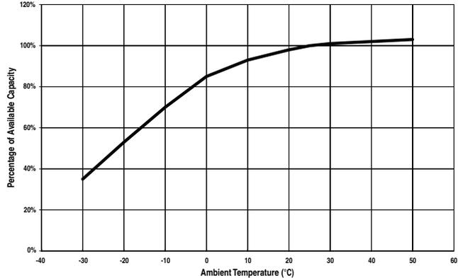
**Capacity vs. Operating Temperatures:** Above are the changes in capacity for wider ambient temperature range, giving the available capacity, as a percentage of the rated capacity, at different ambient temperatures. The curves show the behavior of the battery after a number of cycles.
